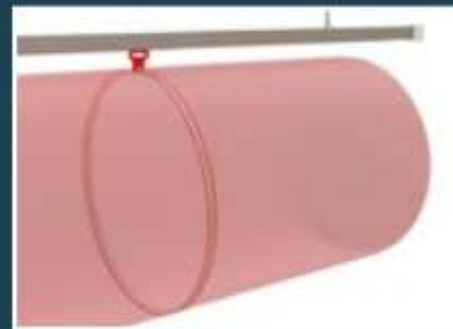
Internal 360° Hoops added to a Type 8 suspension in an internal sleeve
